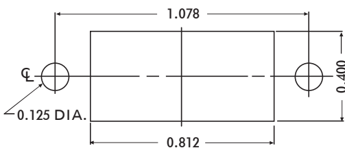
RECOMMENDED CHASSIS CUT-OUT
